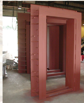
Blast Door Frame Made for Overly Door MFG
